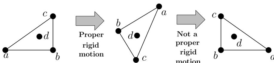
Figure 3: The second transformation is a rigid motion but not a proper one.
